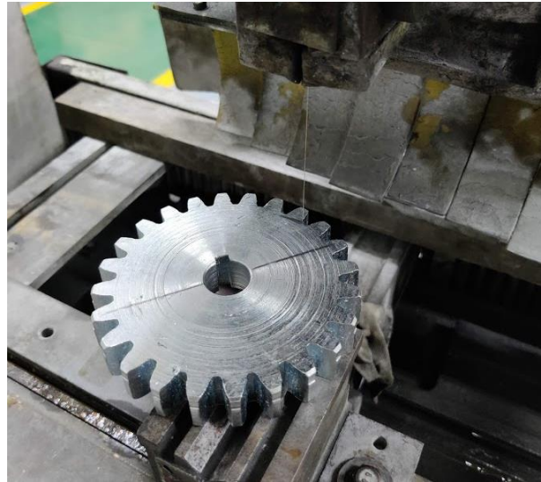
Fig. 2. Wire EDM Cut of Gear
