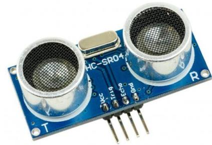
**Fig-4 Ultrasonic Sensor HC-SR04**
