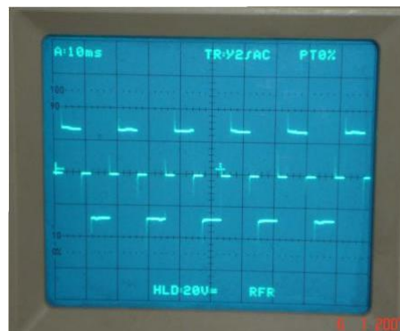
Fig. 12 Result of H-bridge Inverter output ( R_T = 20 \text{ k}\Omega )
