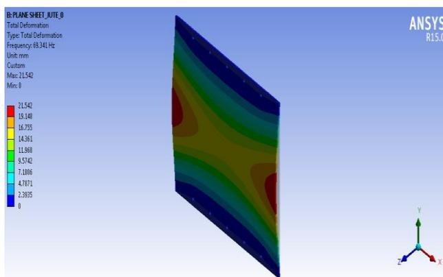
Mode-1. Plane sheet with Reinforcement
