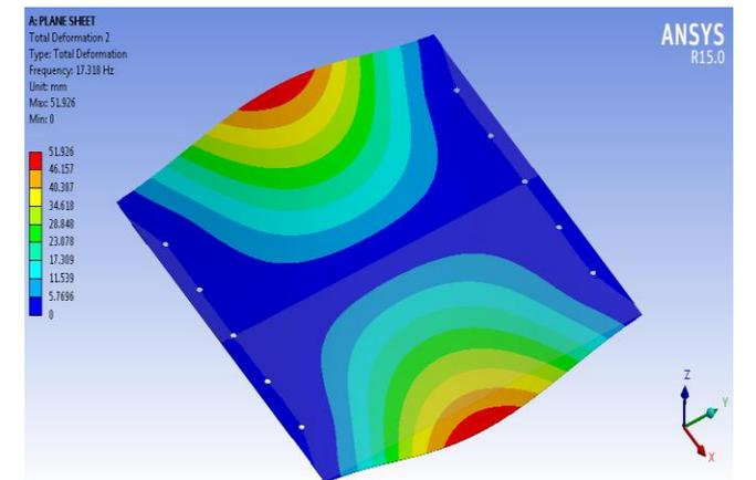
Mode-2. Plane Sheet with reinforcement.
