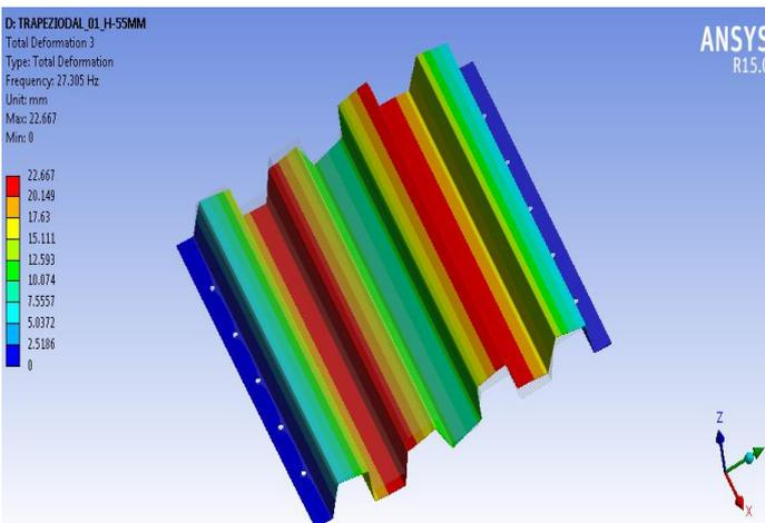
Mode-3. Trapezoidal Sheet with reinforcement.
