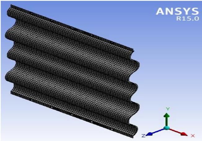
Meshing of Circular with reinforcement
