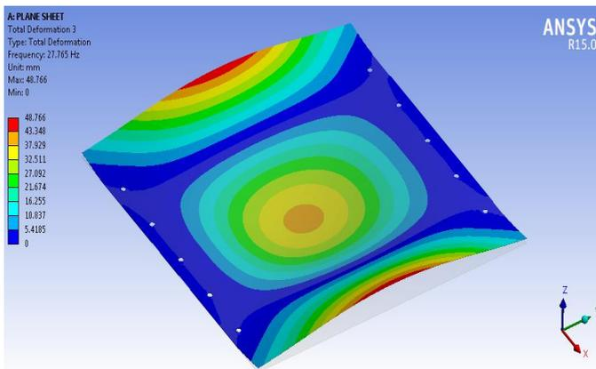
Mode-3. Plane Sheet with reinforcement.
