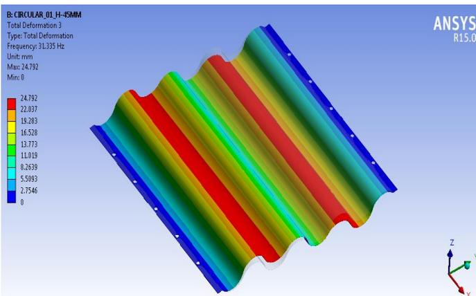
Mode-3. Circular Sheet with reinforcement.
