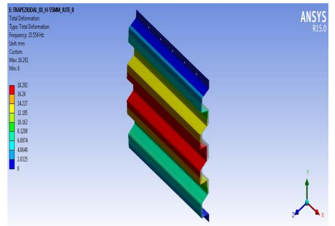
Mode-1. Trapezoidal Sheet with reinforcement.
