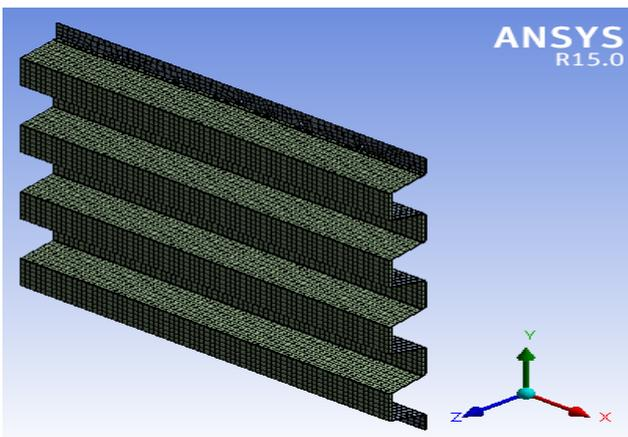
Meshing of Trapezoidal with reinforcement.
