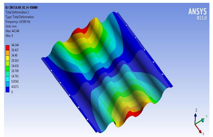
Mode-2. Circular Sheet with reinforcement.
