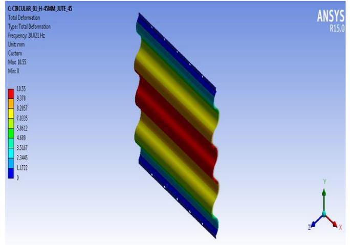
Mode-1. Circular Sheet with reinforcement
