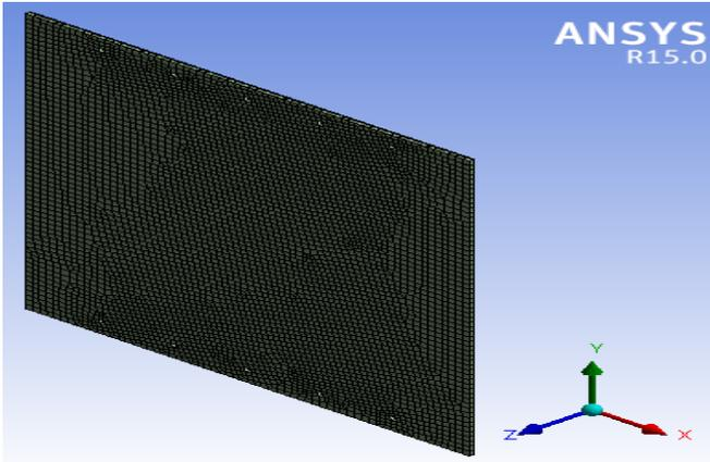
Meshing of Plane sheet with Reinforcement
