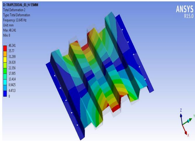
Mode-2. Trapezoidal Sheet with reinforcement.
