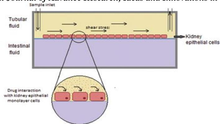
**Fig 3: Kidney-on-a-chip model [24]**
