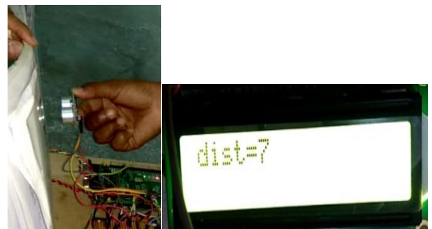
Fig 6. Ultrasonic sensor and object at 7 cm distance which is displaying in LCD
