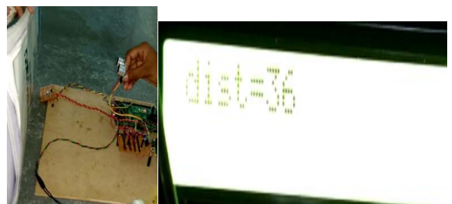
Fig 7. Ultrasonic sensor and object at 36 cm distance which is displaying in LCD
