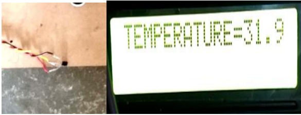
Fig 8. Temperature sensor and LCD displaying surrounding temperature
