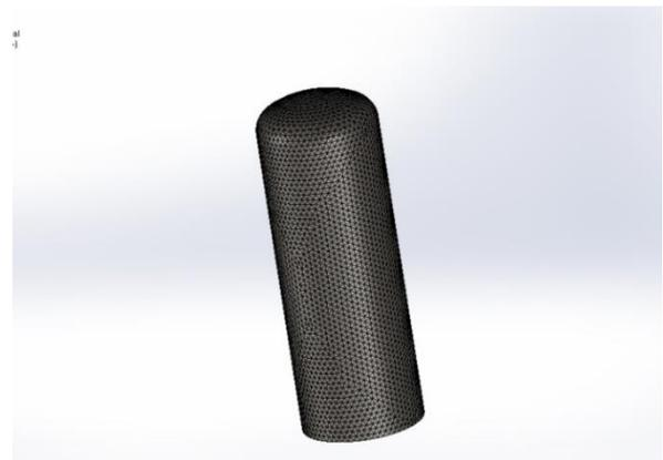
Fig -4: Meshed tank for structural analysis
