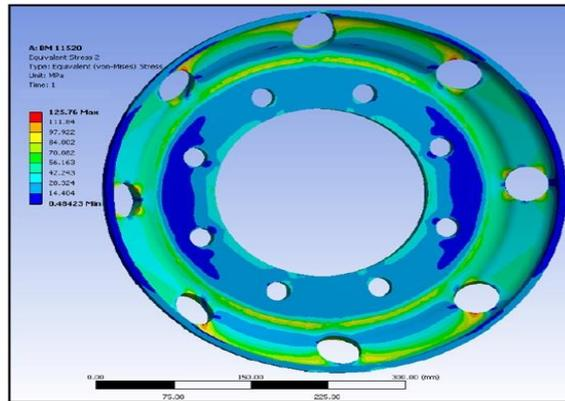
**Fig. 1: Stress plot at 2300kg**
