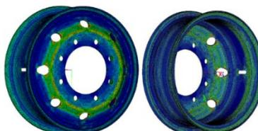
Fig 4.7(b): Bi-Axial Stress distribution in variable Thickness Disc Design
