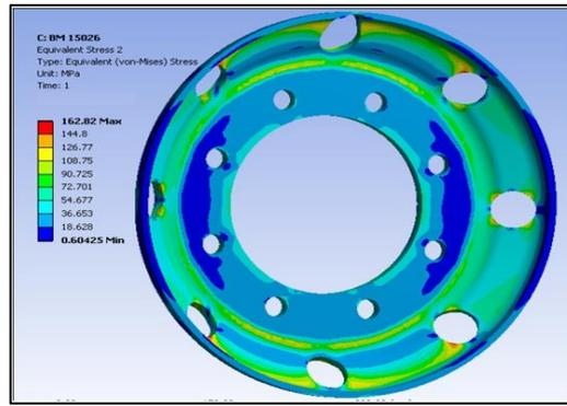
Fig. 3: Stress Plot at 3000 kg
