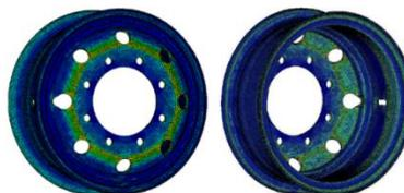
Fig 4.7 (a): Bi-Axial Stress distribution in Uniform thickness Disc design
