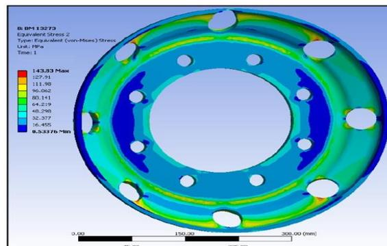
**Fig. 2: Stress Plot at 2600 kg**
