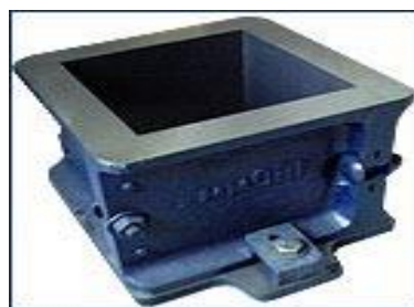
Figure 2: Cube concrete Mould
