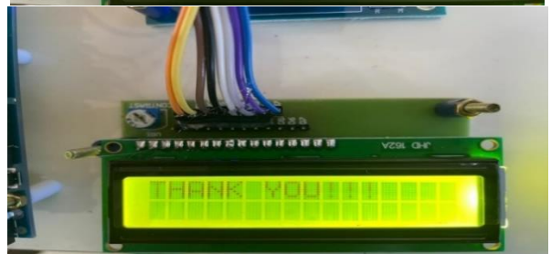
Figure 9 : If user is found unauthorised buzzer goes on..Finally, before logging out it shows "Thank you"
