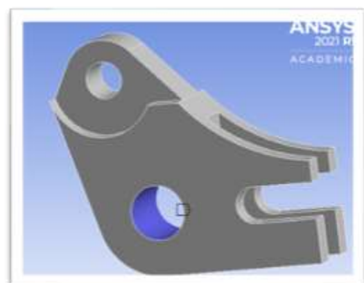
Fig. 2.2: Fixed support is applied at blue part of Toggle Lever
