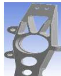
Fig. 1: Shows the 3D model of knuckle
