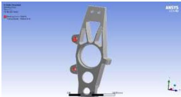
Fig 3: Shows the braking support with 1500 n load.
