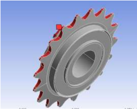
Fig. 2.3: Force of 1000N is applied at red part of Sprocket
