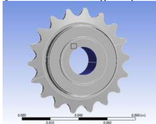
Fig. 2.2: Fixed support is applied at labelled part of Sprocket
