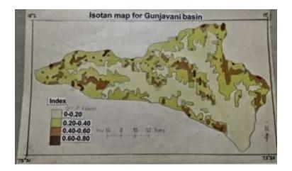
Gradient is always expressed as a ratio between the difference of the maximum and minimum and horizontal equivalent. After finding out the slope of every square of the map showing the lines joining equal value of tangent is drawn which is equal as station map this method was proposed by Miller and therefore it is called as Millers isotan map.
