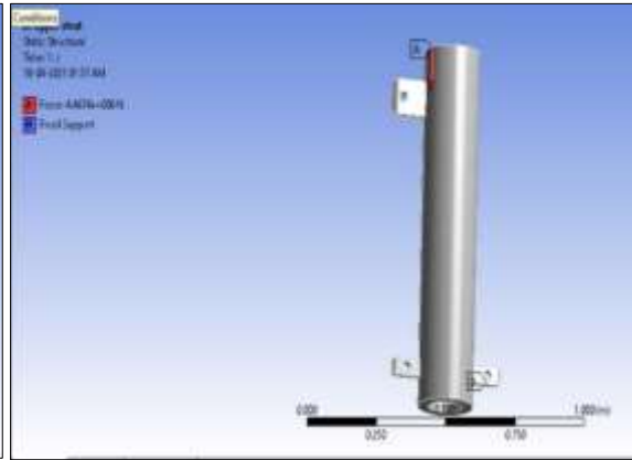
Fig. 06: Load and Fixed Support
