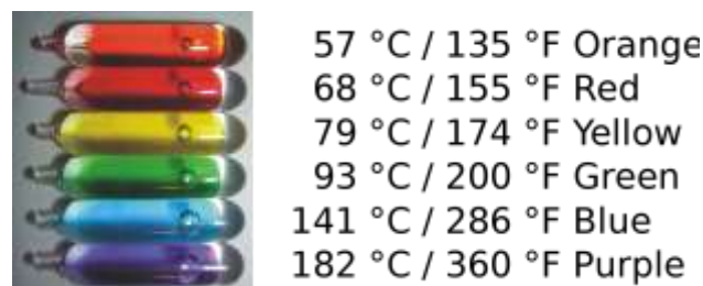
Fig. 1: Types of glass bulb with respective threshold temperature.
