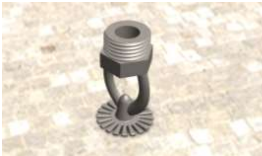
Fig. 2: Water sprinkler design with SOLIDWORKS 2018
