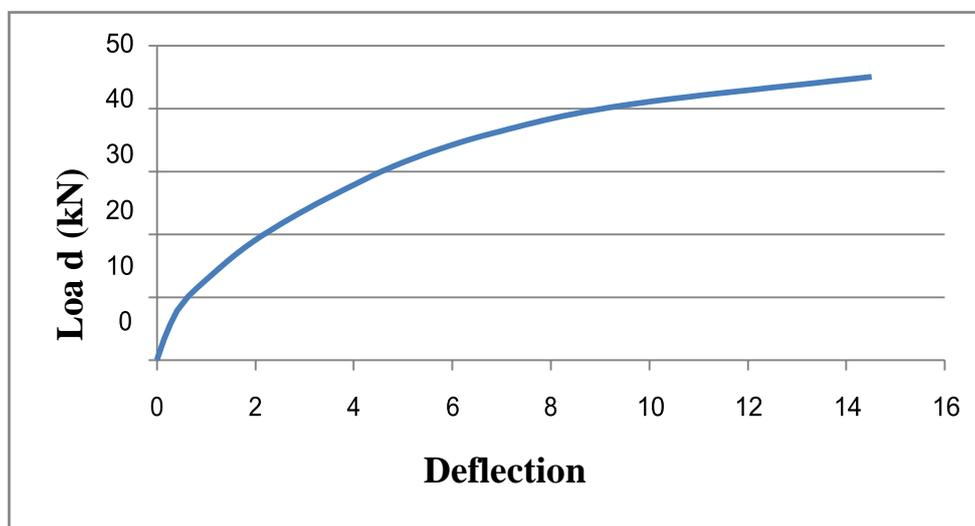
**Graph 1: Load Vs Deflection Curve for Conventional Concrete**
