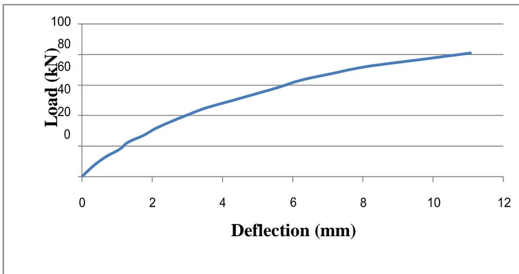
Graph 2: Load Vs Deflection Curve for beam wrapped with basalt fiber fabric
