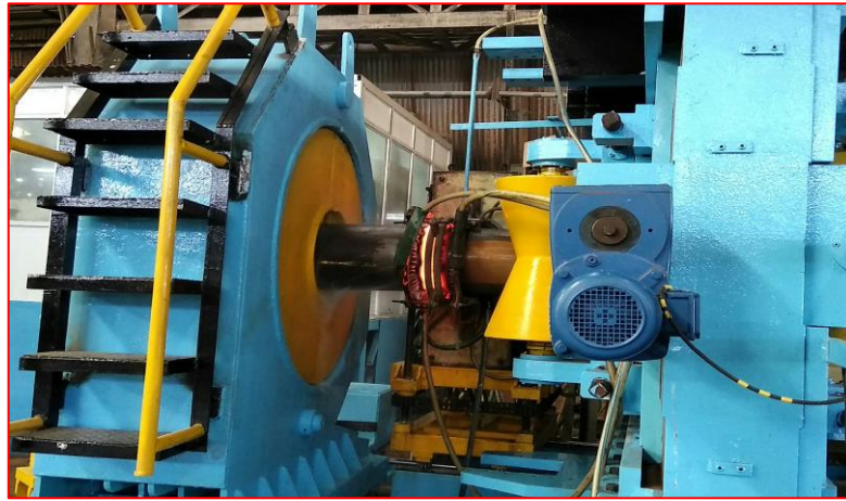
Fig. 1: Hot Induction Bending Process at Jindal Saw Limited, Samaghogha, India
