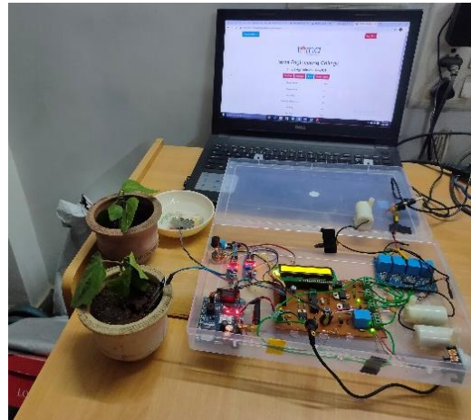
Fig. 1: Experimental setup (interfacing microcontroller, sensors, relay, and motor pump)
