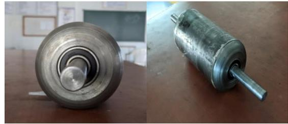
Fig. 21: Fabricated Roller - info [2.2.1]
