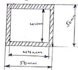
Fig. 17: Cross-section of frame
