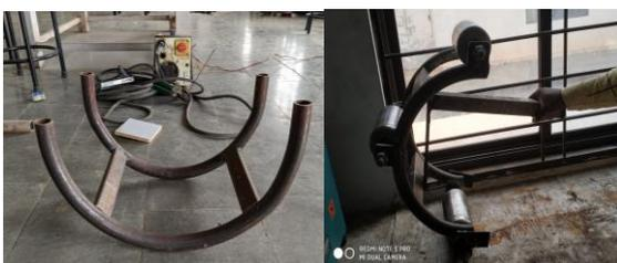
Fig. 20: C- Frame Chassis after fabrication -info [2.2.2]
