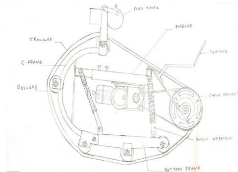
Fig. 2: Schematic View of Mono bike
