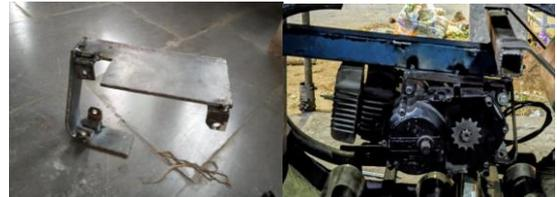
Fig. 22: Fabricated Engine Frame-info [2.2.4]
