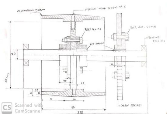
Fig. 7: Transmission Drum
