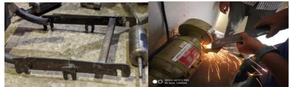
Fig. 23: Fabricated Bottom Chassis Frame – info [2.2.5]
