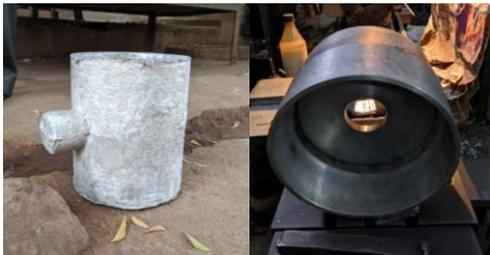
Fig. 19: Transmission Drum After Casting And lathe operations
