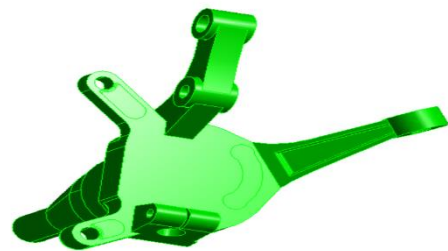
2. Material removal from the longer arm
