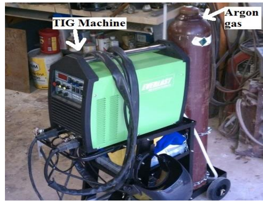
Fig. 2: TIGWelding Setup– Ever Last TIG 250 AC/DC TIG Welding System
