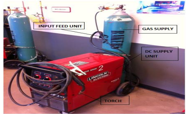
Fig. 3: Image of MIG Welding System Welding Setup
