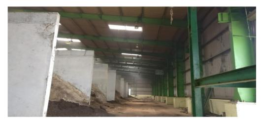
The RDF stored at front side of the plant was engulfed by fire since two days. 20 to 30 tones of RDF and dry garbage was burning with smoke. Previous day they douse it by fire engine. When expert visited to the spot we removed few layers of garbage and douse it and douse fire balls. Inside the plant windrows pads were also about to catch fire for precautionary step they poured water to not catch fire. RDF was stored in plant B and almost 40 to 50 tons burnt and ashes were found.
