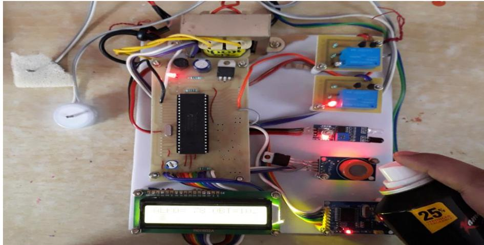
Fig. 3: Alcohol sensed by the sensor
