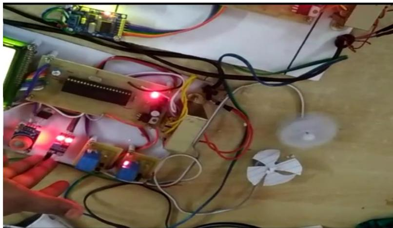
Fig. 4: Automatically Break Apply when obstacle comes near to vehicle.
