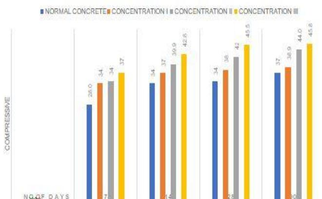
**Fig. 4: Bar chart of compressive strength**
