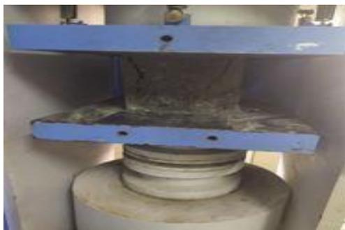
Fig. 5: Compression test of cube
