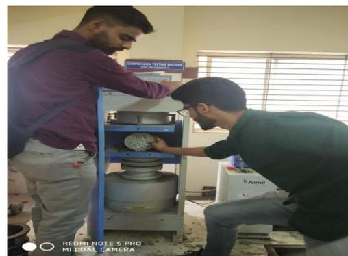
Fig. 14: Testing of Cylinders
