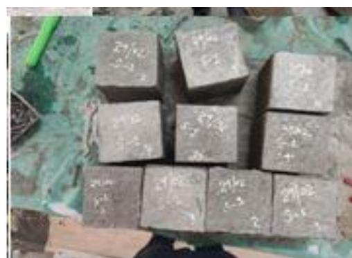
Fig. 16: De-moulding of Cubes
