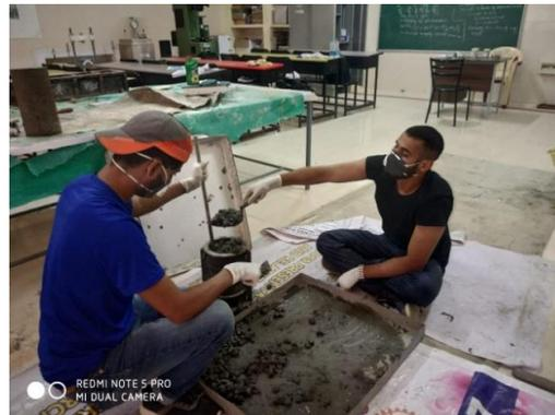
Fig. 13: Casting of Cylinders
