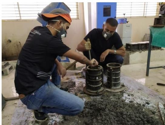
Fig. 9: Casting of Cylinder
