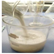
Fig. 7: Adding GBFS to diluted acid
