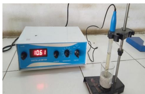
Fig. 5: pH value of Crushed GBFS
