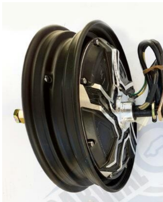
Fig. 5: 48V/800W BLDC Hub Motor [10]
