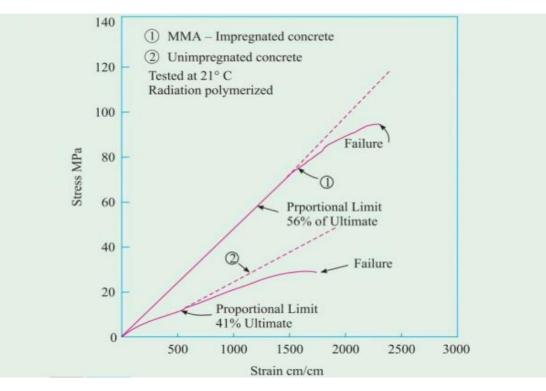
PIC has linear stress-strain relationship up to 80% of ultimate strength and there is no abrupt change at proportional limit. The stress strain curves for Styrene-TMPTMA impregnated concrete also show the same characteristics as MMA impregnated concrete.
