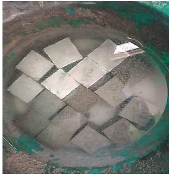
Fig. 8: Curing of cubes
