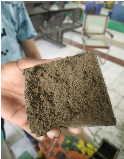
Fig. 10: After test broken piece of mortar cube
