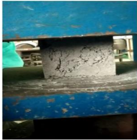
Fig. 9: Testing of Cubes
