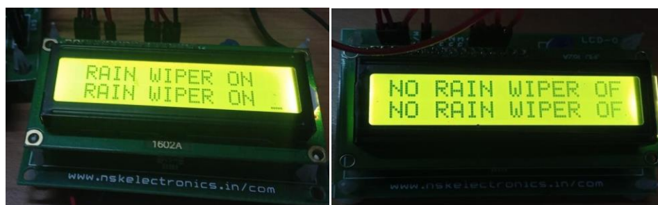
Fig. 3: Wiper control system in rain condition and no rain condition
