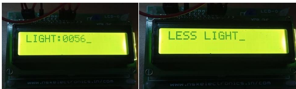
Fig. 2: Darkness level monitor for headlight operation
