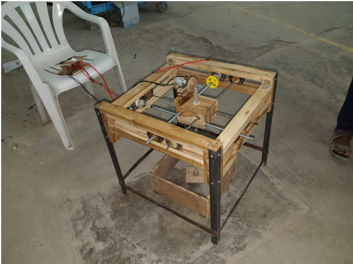
Fig. 14: Old version of our motor operated automatic ramming machine
