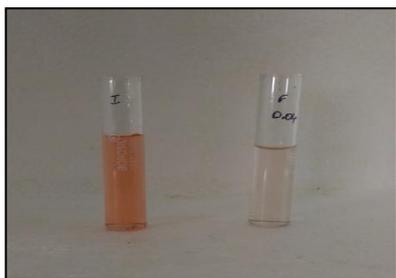
**Fig. 6: Decolourization of Congo red solution at 0mins and 60mins**
