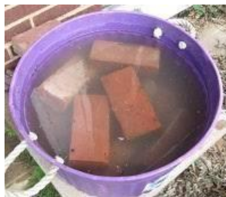
Fig. 6: Water Absorption test
