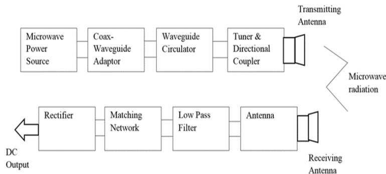
**Fig. 1: Block Diagram of Microwave Power Transmission System**
