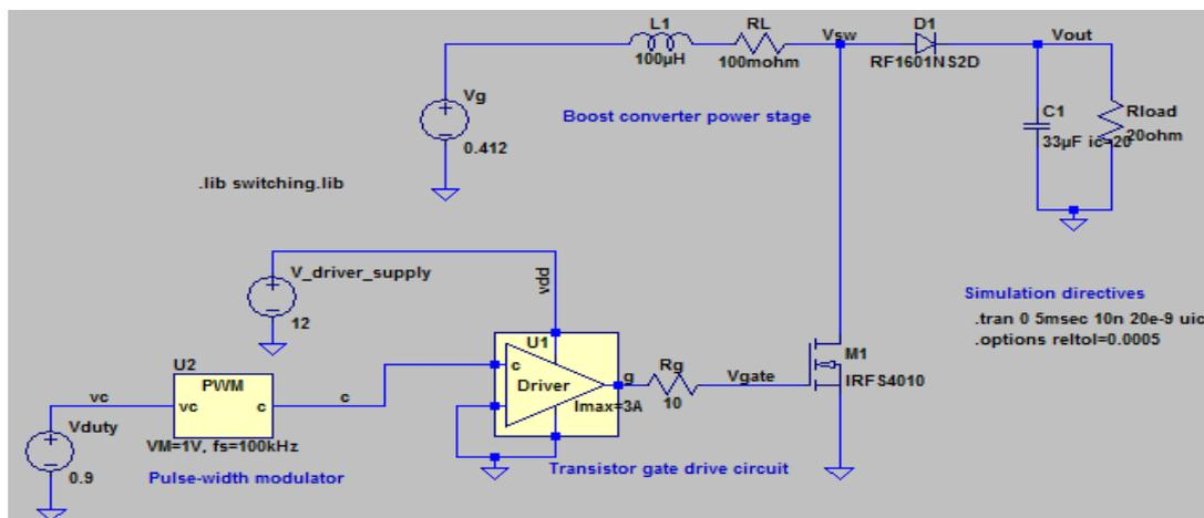
Fig. 3: Schematic diagram of boost converter
