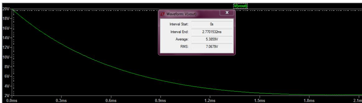
Fig. 4: Output waveform of boost converter
