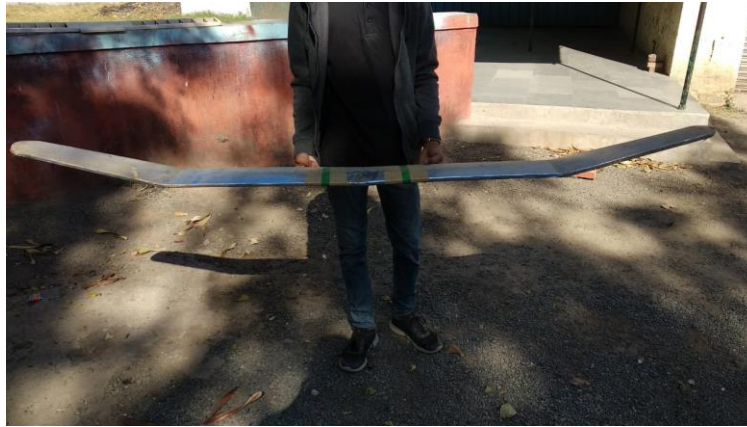
Fig. 7: Manufactured Tip Dihedral Wing
