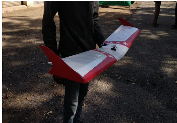
Fig. 5: Manufactured Dihedral Wing
