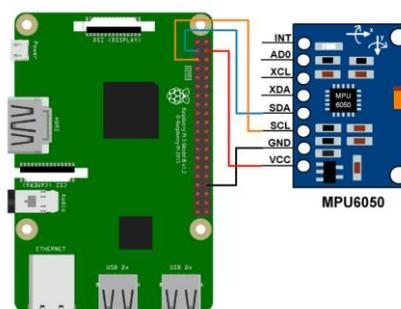
**Fig. 2: IMU Connection to Raspberry-pi**
