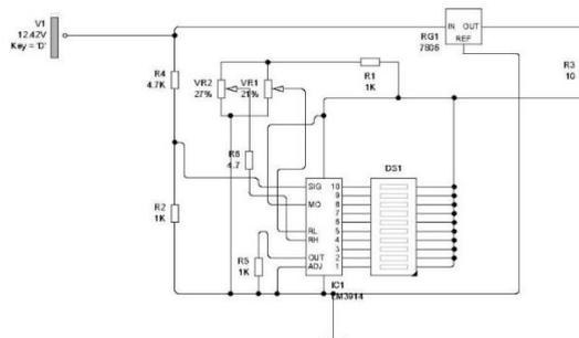
**Fig. 7: Simulation circuit of Battery Level Indicator**
