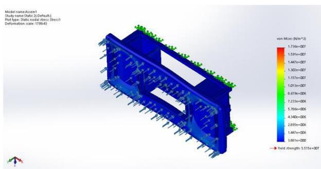
Fig. 10: Stress analysis of the Hover-board
