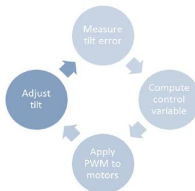
**Fig. 5: Balance Algorithm**
