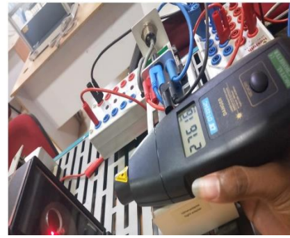
Fig. 4: Reading RPM using tachometer
