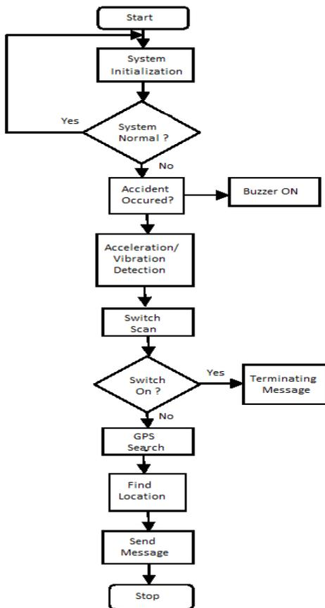
Fig. 5: Flow chart of Automatic Vehicle Accident Detection and Rescue System
