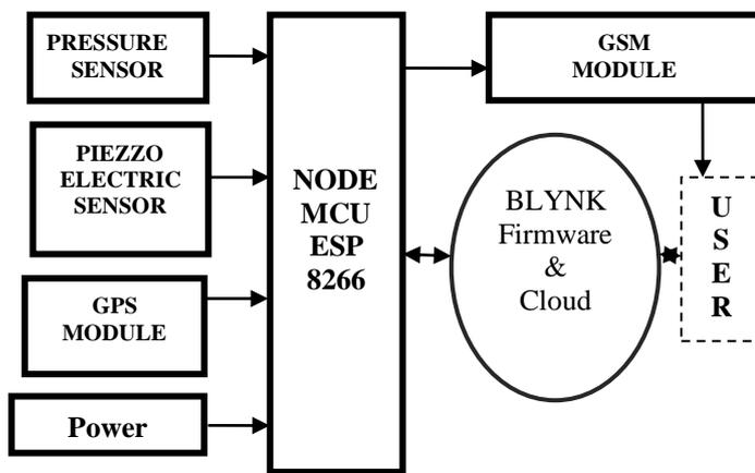
Fig. 1: Block diagram of Automatic Vehicle Accident Detection and Rescue System
