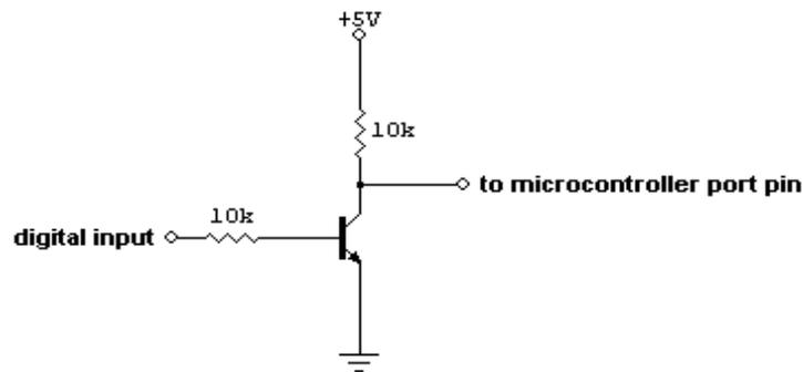
Fig. 3: Switch Circuit
