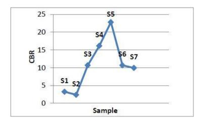
By increasing the red mud up to 40% to the soil with 3% lime, the best results were come out at 20% red mud soil mixture. At this proportion the MDD and CBR value increases up to 1.811g/cc and 22.81% respectively at OMC of 17.50%.
