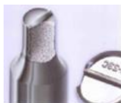
Fig. 6: Punch Tip Cup Breakage
