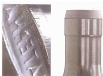
Fig. 8: Tip Wear by abrasion
