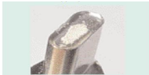
Fig. 3: Product sticking to the face of an upper punch
