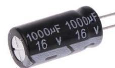
**Fig. 4: 1000µF capacitor (Used as Filter)**
