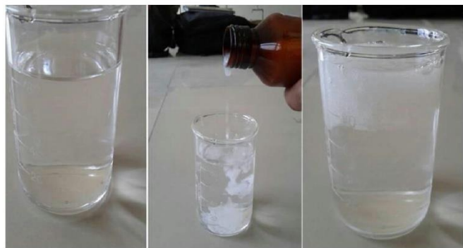
Fig. 10: Gelling behaviour of (a) F9 formulation (b) Formation of stiff gel.
