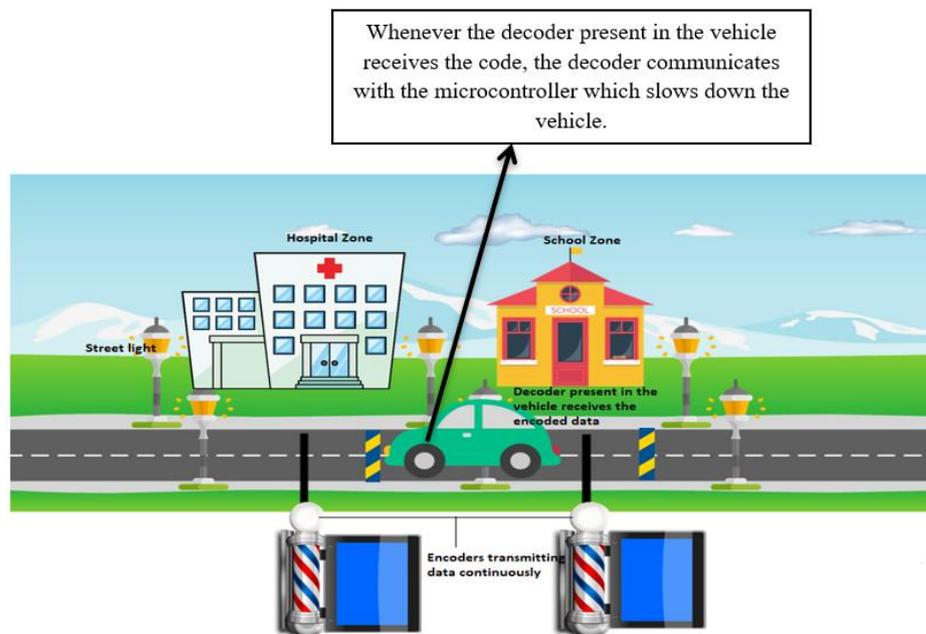
Fig. 9: Working procedure-using encoders and decoders
