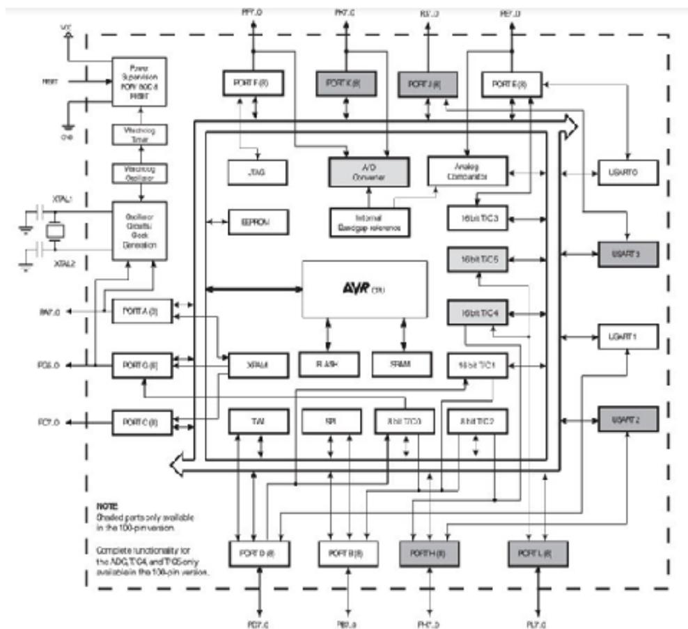
Fig. 2: Architecture of AVR microcontroller
