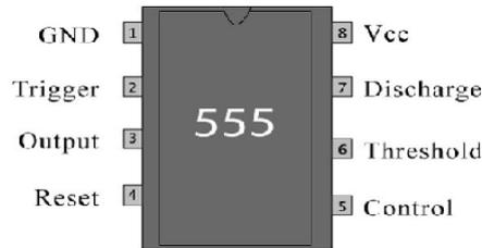
Fig. 3: 555 Timer pin diagram
