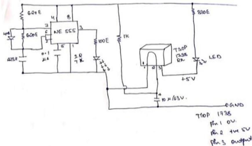
Fig. 13: Circuit diagram for object detection sensor diagram
