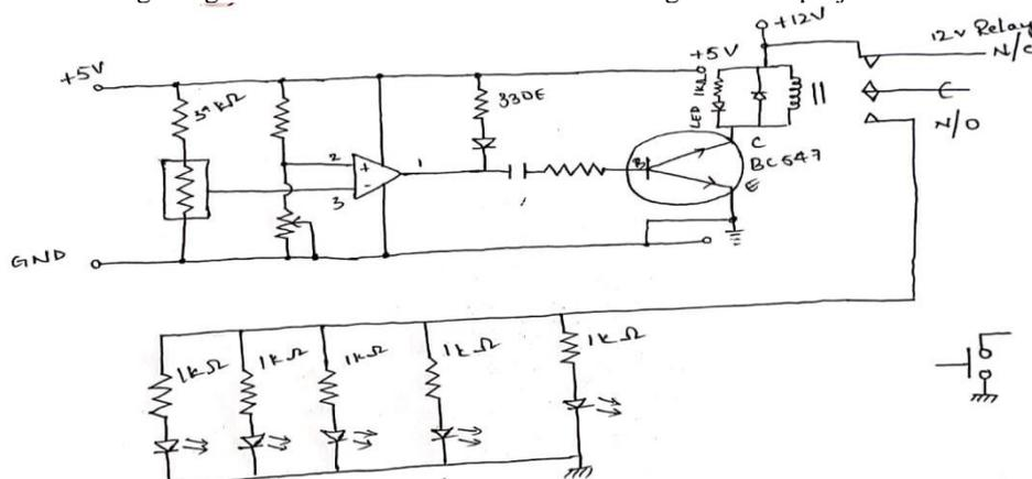
Fig. 14: Circuit diagram for street light
