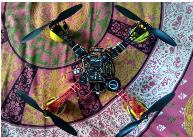
Fig. 1: Our quad after mounting the motors and essential components
