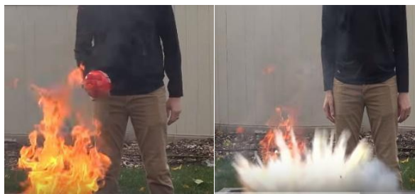
Fig. 4: Image of extinguishing fire using ABC fire ball
