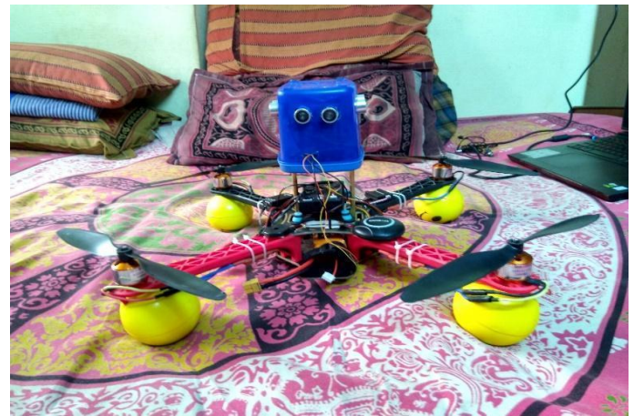
Fig. 2: The quad with the UNO and collision avoidance system on top of FC
