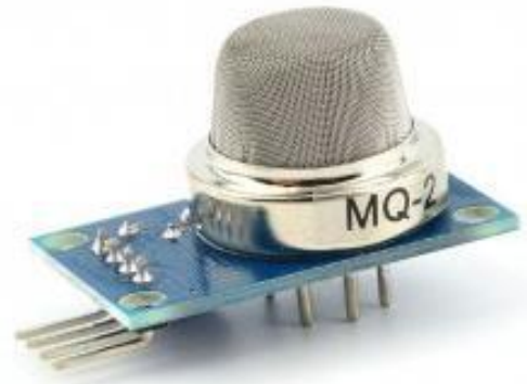
Fig. 4: MQ-2 (Hydrocarbon Sensor)
