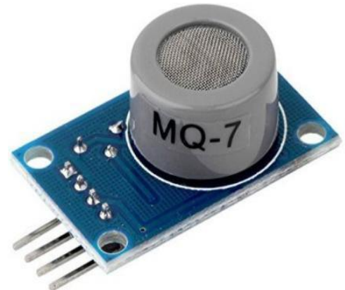
Fig. 5: MQ-7 (Carbon Monoxide Sensor)
