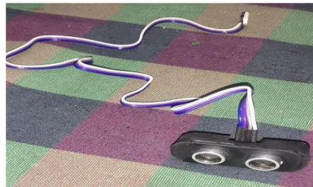
Fig. 9: Ultra Sonic Sensor
