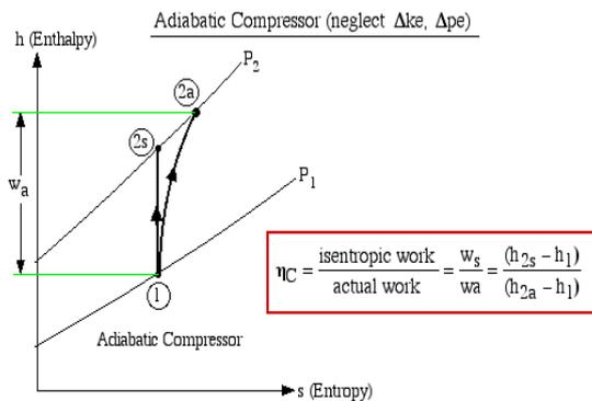
Fig. 1: H-S dia. For compressor
