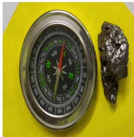
Fig. 6: Unknown iron meteorite placed near Mariner compass. No deflection of the needle
