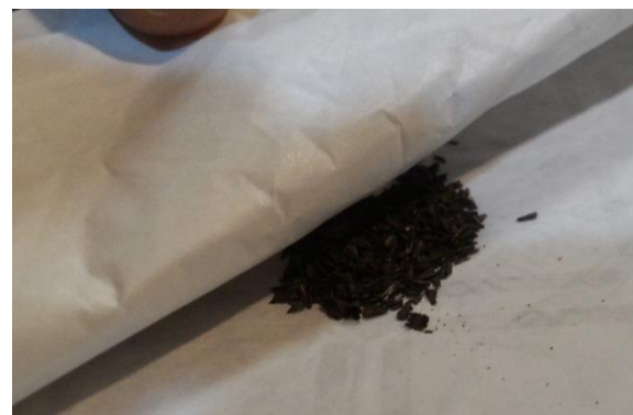
Fig. 20: A stony meteorite wrapped in a butter paper and gently rolled over iron filings to study the magnetic property. No movement or attraction of iron filings towards a meteorite observed
