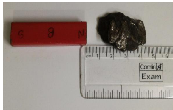
Fig. 23: Measuring the distance of attraction of an iron meteorite Campo-del-Cielo (2), towards a bar magnet
