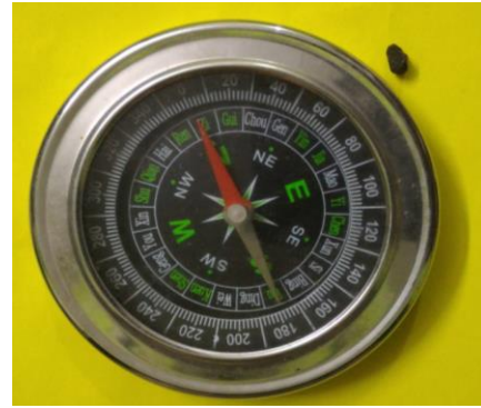
Fig. 8: Chelyabinsk stony meteorite placed near Mariner compass. No deflection of the needle
