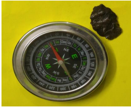
Fig. 7: Campo-del-Ceilo (2) iron meteorite placed Mariner compass. No deflection of the needle
