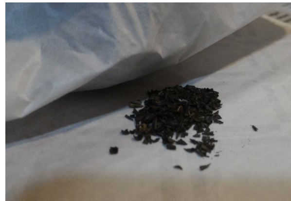
Fig. 18: An iron meteorite wrapped in a butter paper and rolled gently over iron filings to study the magnetic property. No movement or attraction of iron filings towards a meteorite observed
