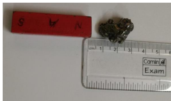
Fig. 25: Measuring the distance of attraction iron meteorite Sikhote Meteorite Campo-del-Cielo (1) towards a bar magnet
