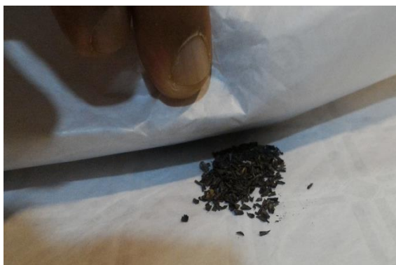
Fig. 19: An iron meteorite wrapped in a butter paper and gently rolled over iron filings to study the magnetic property. No movement or attraction of iron filings towards a meteorite observed
