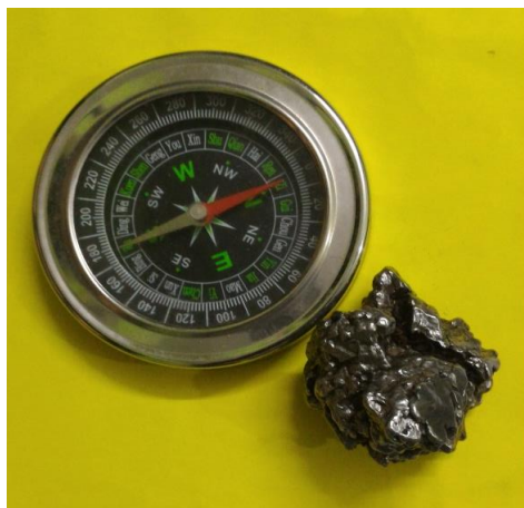
Fig. 5: Unknown iron meteorite placed Near mariner compass. No deflection of the needle
