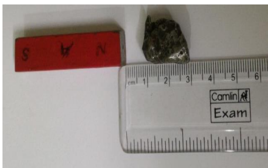
Fig. 24: Measuring the distance of attraction of an Alin towards a bar magnet
