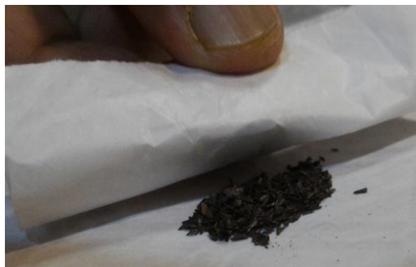
Fig. 21: An iron meteorite wrapped in a butter paper and gently rolled over iron filings to study the magnetic property. No movement or attraction of iron filings towards a meteorite observed
