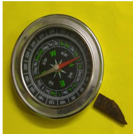
Fig. 4: Unknown iron meteorite placed near Mariner compass. No deflection of the needle
