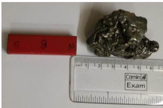
Fig. 22: Measuring the distance of attraction of an Unknown iron meteorite (2), towards a bar magnet
