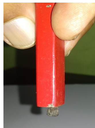
Fig. 14: Chelyabinsk stony meteorite strongly attracted towards a bar magnet
