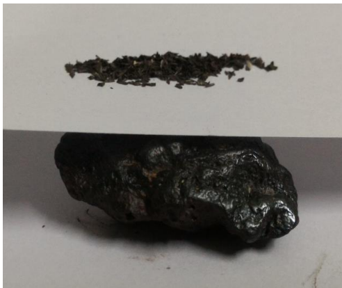
Fig. 17: Iron filings held over the unknown iron meteorite to find the magnetic property. No movement of iron filings observed
