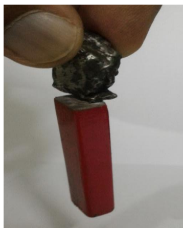
Fig. 13: Sikhote Alin iron meteorite strongly attracted towards a bar magnet
