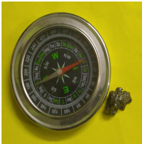
Fig. 3: Campo-del-Ceilo (1) iron meteorite placed near Mariner compass. No deflection of the needle
