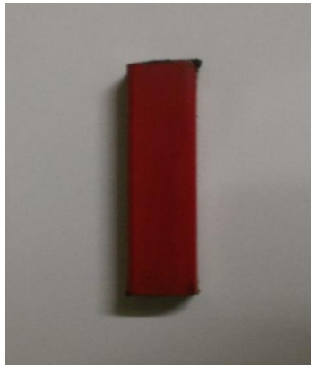
Fig. 9: A plain bar magnet used to find attractive Property of meteorites
