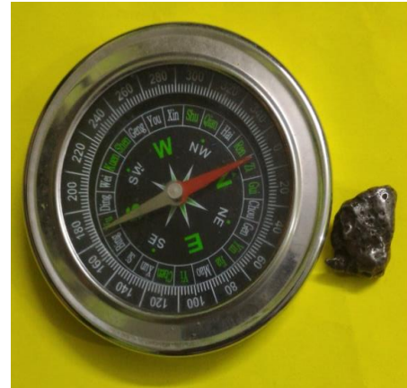
Fig. 2: Sikhote Alin Iron meteorite placed near mariner compass. Showing no deflection of the needle
