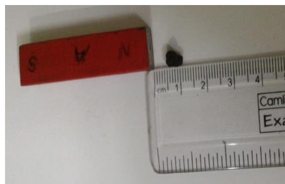
Fig. 27: Measuring the distance of attraction of a Stony meteorite Chelyabinsk towards a bar magnet
