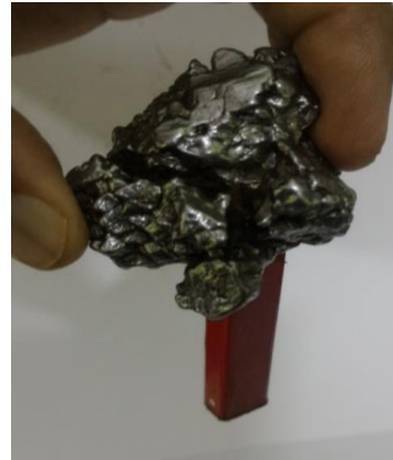
Fig. 10: Unknown iron meteorite strongly attracted towards a bar magnet
